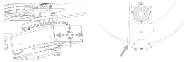
IMPORTANT: Moving the limit switch too far left may prevent the clay from falling onto the sliding plate in time and causing it to break. Moving the limit switch too far right may cause the throwing arm to not stop and the motor to run continuously.
