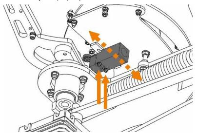
To properly adjust the limit switch, loosen the two nuts and move the switch so that the throwing arm stops at the proper location. Remember, that moving the limit switch to the left will stop the throwing arm earlier, and moving it right will stop the throwing arm later.
